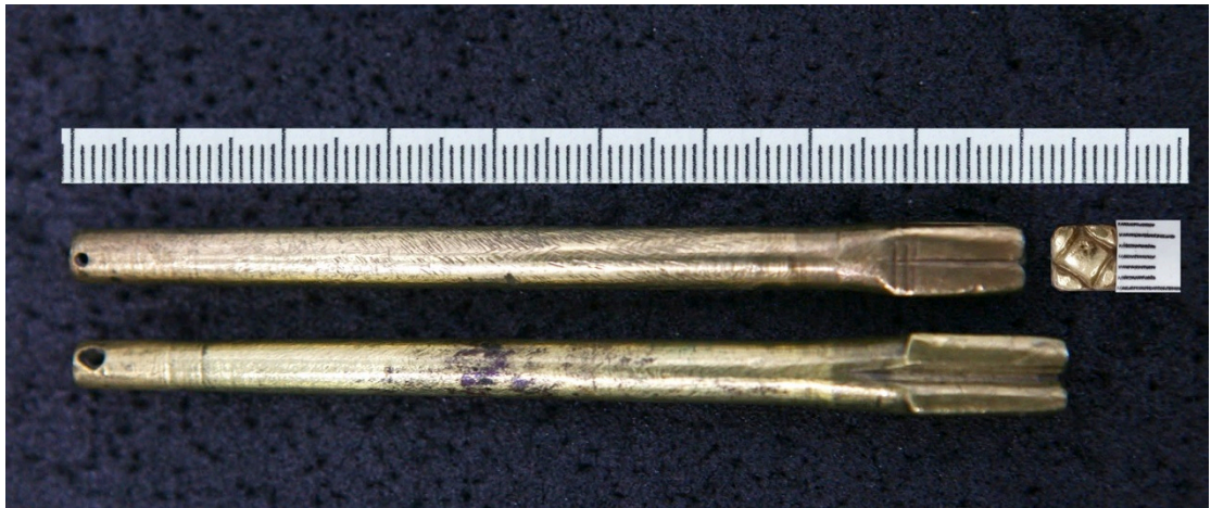
Figure 3.23: two different Lamont harp tuning pins. Pin #11 (top) from Group A, and pin #22 (bottom) from Group C. In addition to the differing designs of the drive heads, the lengths, and the colour of the alloy are also different. The scale is 1 tick : 1 mm.
