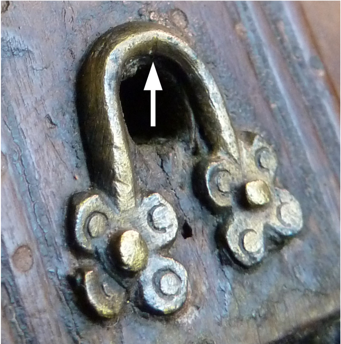
Figure 3.65: shoe at string hole #32 of the Lamont harp. There is a single light mark (arrowed), possibly from a wire string. The shoe at string hole #31 has a similar mark in the same location. The position of this mark is consistent with the use of this string hole with the forepillar pulled over towards the left side of the instrument, as it is currently.
